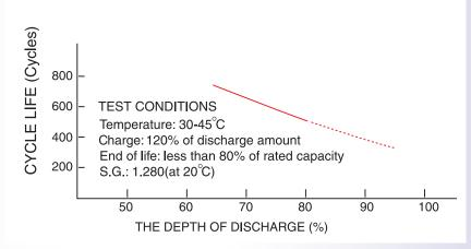
Life of batteries is mostly affected by the depth of discharge. Repetition of deep discharge makes the life of batteries shorten.
