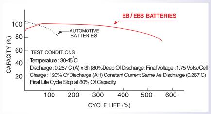
As designed for cyclic services having 4 times longer life than automotive batteries.
